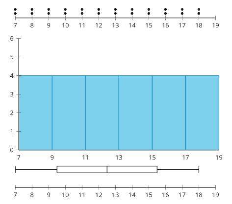
In a uniform distribution the mean is equal to the median since a uniform distribution is also a symmetric distribution. The box plot does not provide enough information to describe the shape of the distribution as uniform, though the even length of each quarter does suggest that the distribution may be approximately symmetric. A **bimodal distribution** has two very common data values seen in a dot plot or histogram as distinct peaks.
