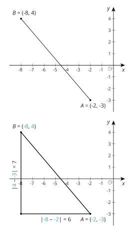
The length of the horizontal leg is 6, which can be seen in the diagram, but it is also the distance between the *x*-coordinates of *A* and *B* since |-8 - -2| = 6. The length of the vertical leg is 7, which can be seen in the diagram, but this is also the distance between the *y*-coordinates of *A* and *B* since |4 - -3| = 7.
