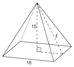
a. What is the measurement of the slant height  $\ell$  of the triangular face of the pyramid? If you get stuck, use a cross section of the pyramid.
